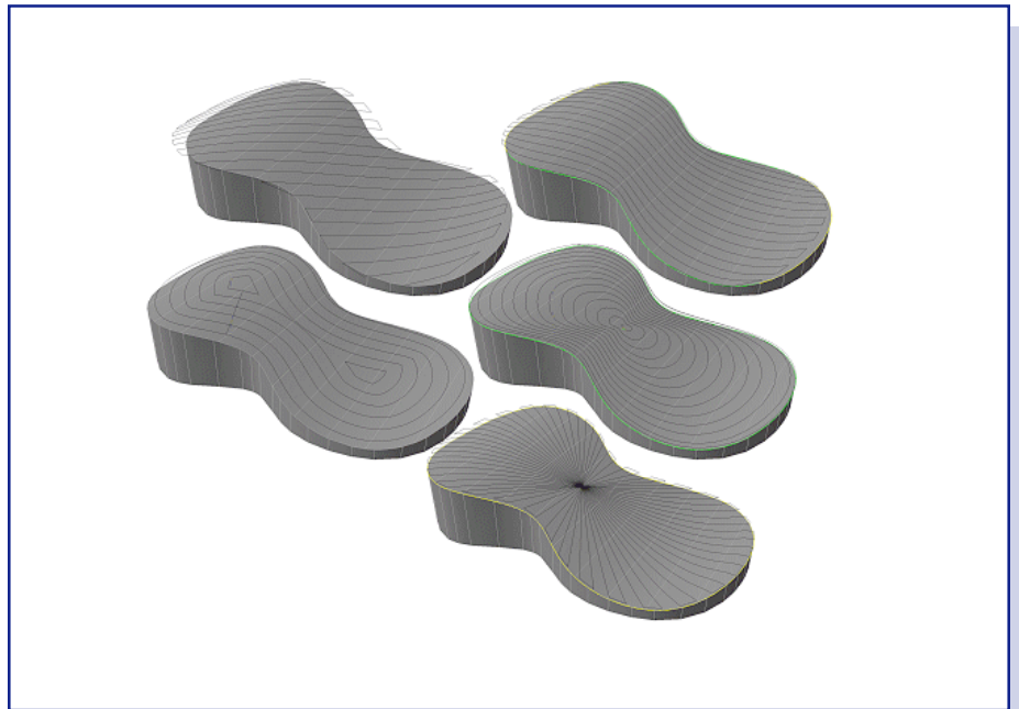
I-DEAS Generative Machining provides a variety of cutting patterns for surface machining.
